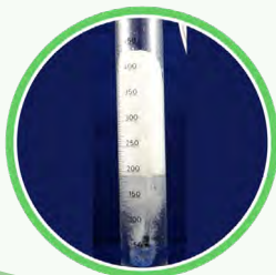
Foaming before addition of Dfoam
