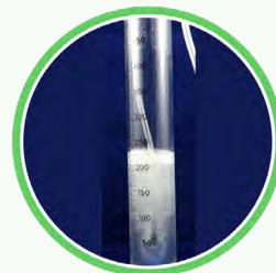
Foam control during aeration after Dfoam added
